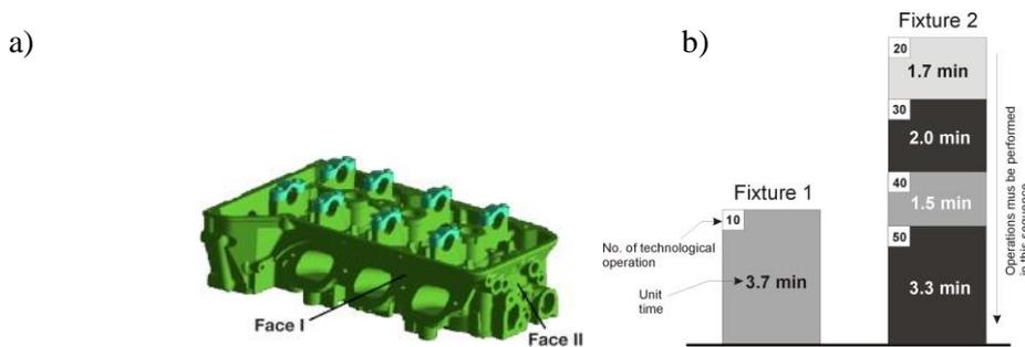
**Fig. 2. Casing-class part to be manufactured in RMS: a) general schematic view of the product, b) structure of the product's technological process [16]**
