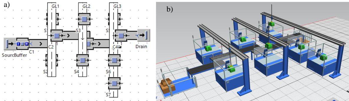
**Fig. 4. Example of simulation model for configuration B developed using Tecnomatix Plant Simulation software: a – 2D model; b – 3D model**
