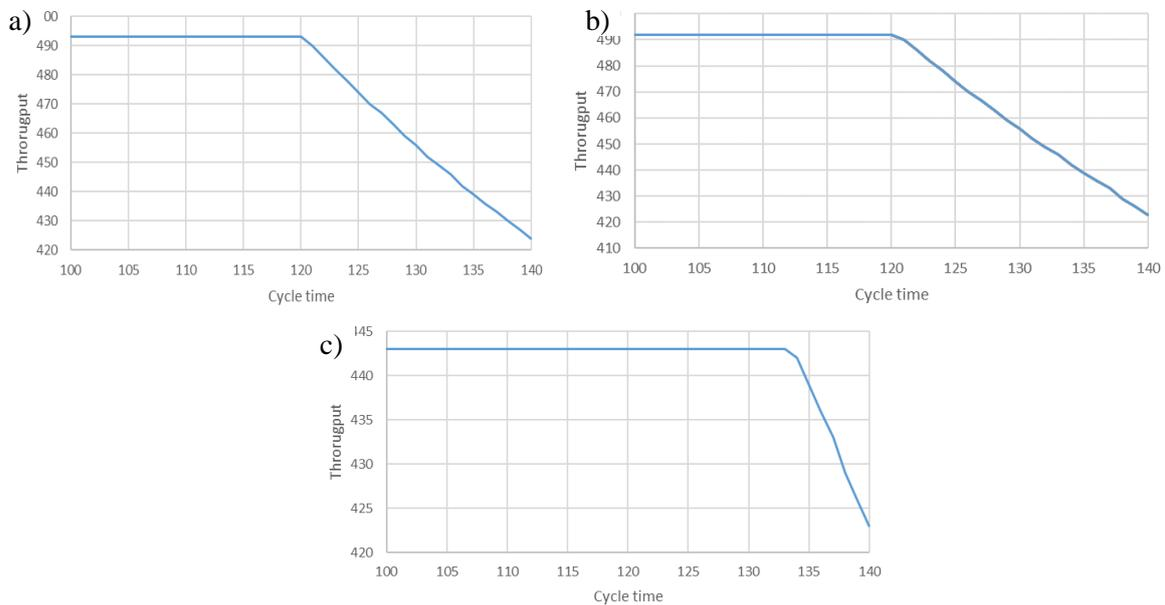
Fig. 5. Relationship between cycle time and throughput of RMS: a – for configuration A; b – for configurations B,C,D,F,G; c – for configurations E and H
