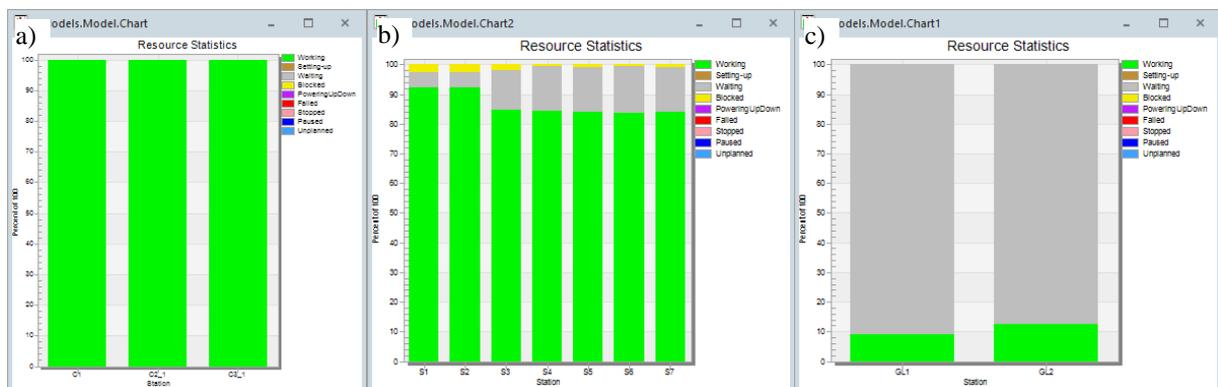
Fig. 6. Level of usability of particular elements of designed RMS for configuration A with defined cycle time of 120 s: a) conveyors, b) machine tools, c) gantries
